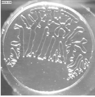
Figure 5: typical image of the debonding of the adhesive from the low adhesion surface. The bottom part of the probe is not in contact.
